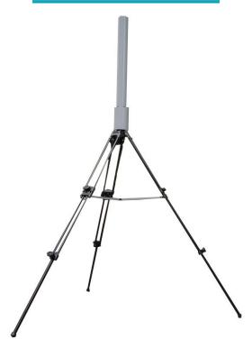
**WxAS-101** is a set of Antennas for Upper air Sounding, It is possible to receive the frequency of  $400 \sim 406 \text{MHz}$  and the receiving distance is 150km. The preamplifier is built in, and the length of the accessory antenna connection cable is 30 m.
