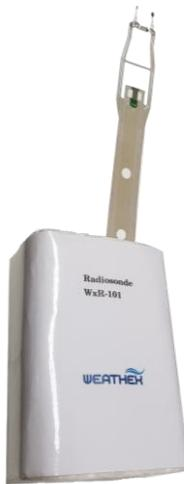
The WxR-101D uses Upper air meteorological simulation system to precisely calibrate according to wind speed and solar radiation in various weather conditions, and has high observation accuracy. Dual temperature sensor technology enables real-time correction of solar radiation regardless of visibility, latitude, longitude and sun altitude.
